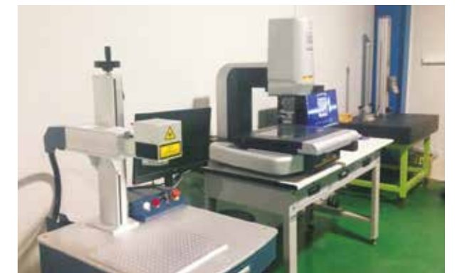
HAXAGON Swiss-made TESA Visio 300 DCC automatic video-based machine, contributing to the quality control of preform molding
