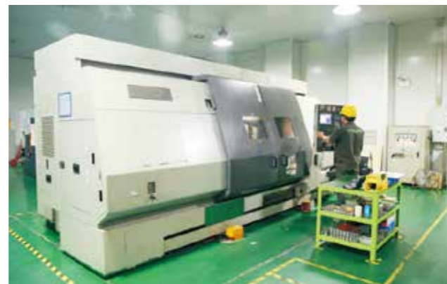
MORI SEIKI 9-axis turning-milling machine, which ensures the cavity parts are formed in one time with high precision
