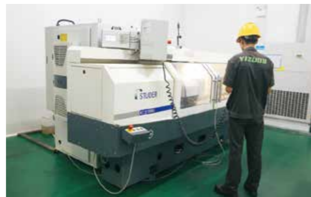
Swiss STUDER CNC universal grinding machine, with precision up to \pm 0.002\text{mm} , ensures precise core taper and extends the mold life. It can also increase the core concentricity so that the preform thickness tolerance is less than \pm 0.02\text{mm} .
