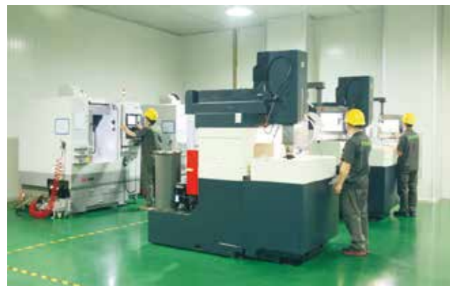
MAKINO electrical die machine and 4-axis CNC engraving and milling machine, which limit the pitch tolerance to \pm 0.005\text{mm}
